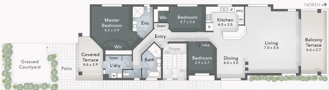
// FLOOR PLAN First Floor - 2.5m Ceiling
