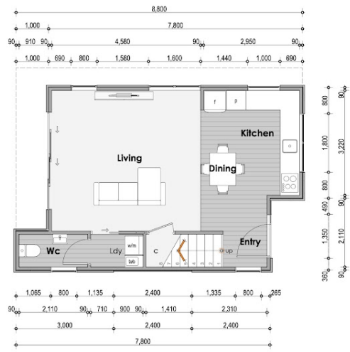
UNIT 1 Ground Floor Area 42.67 m 2
