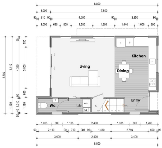
UNIT 2 Ground Floor Area 43.76 m 2
